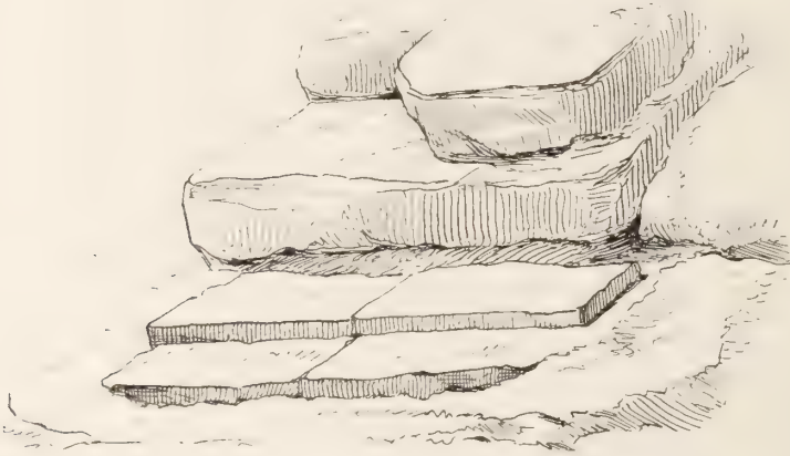
FIG. 49.—Stone substructures of mud wall.
